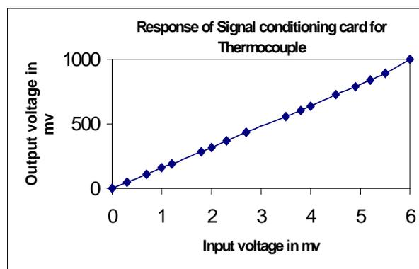
**Figure 6:** Response of Signal Conditioning Card for J-Thermocouple
