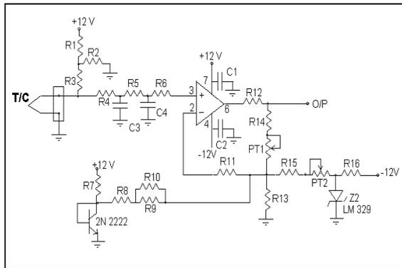
**Figure 1:** Signal Conditioning Circuit for J-Thermocouple
