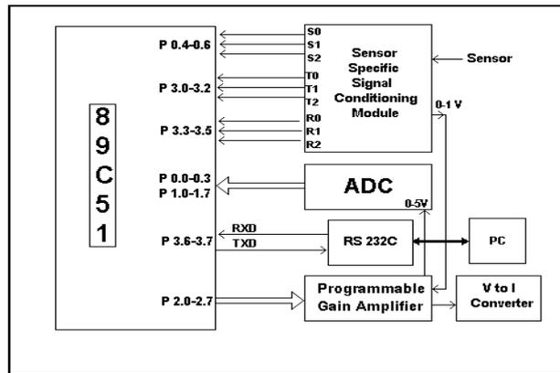
**Figure 3:** Port Configuration of Microcontroller
