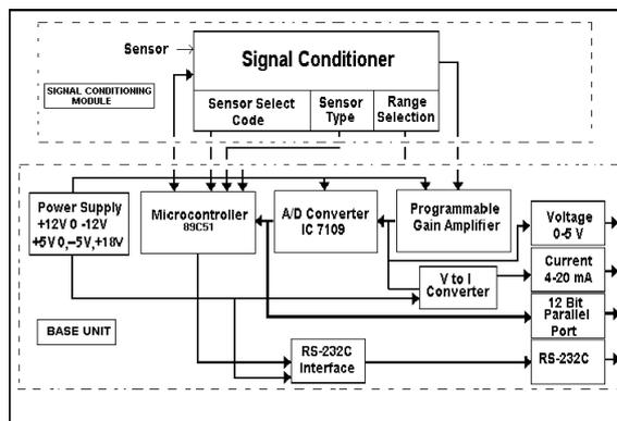
**Figure 2:** Block Diagram of Universal Intelligent Sensor Interface
