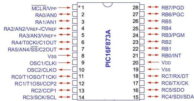
Figure 3. Pin Diagram of PIC16F873A Microcontroller
