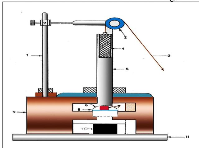
**Figure 1.** Schematic diagram of the experimental arrangement used for measuring ML.
