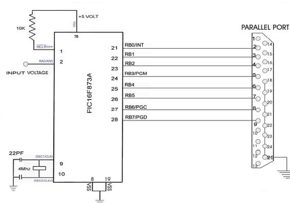
Figure 4. Circuit Design with Port
