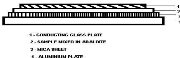
Figure 2. Electrode configuration of an Electroluminescence cell
