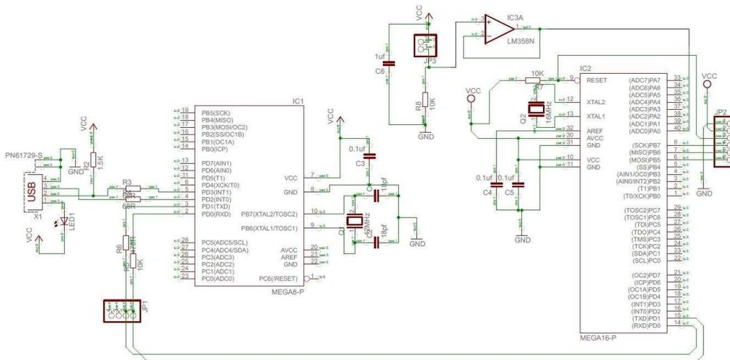
Figure 2. Schematic of the Data acquisition System
