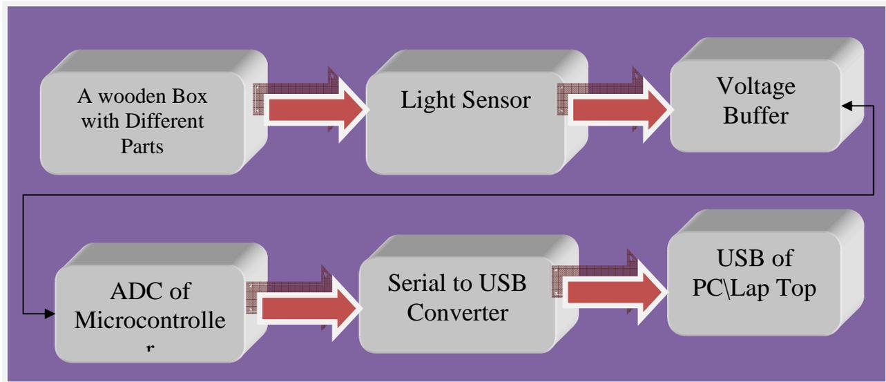
Figure 1. Bloc Diagram of DAQ Device.
