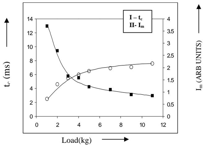
Fig. 3 : Dependence of  $t_c$  and  $I_m$  on the applied load on crystal .
