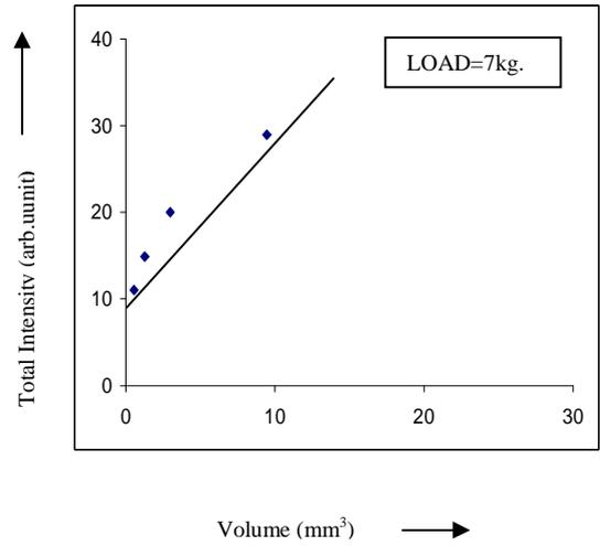
Fig. 2: Dependence of total ML intensity on the volume of crystal
