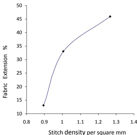
**Figure 1.** The effect of stitch density on fabric extensibility
