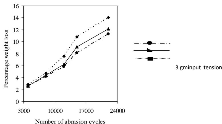
**Figure 2.** Abrasion resistance of the knitted fabric samples
