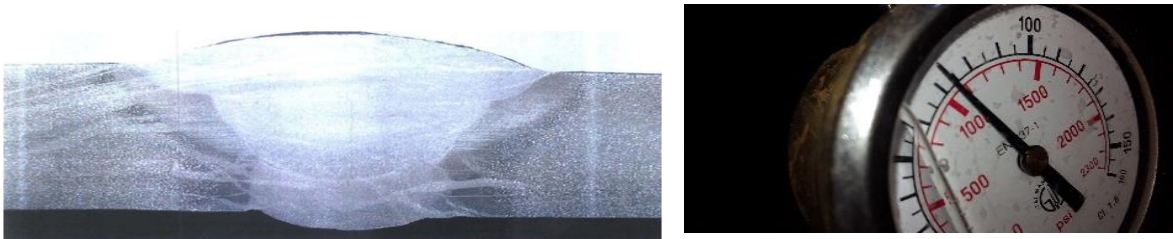
Figure 9: a) X-ray film in the welding joints b) Pressure during the test at the quota 1920m asl (124 bar)
