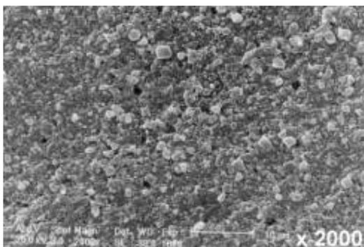
Fig 3. SEM of microfilled hybrid composite (M. Spillers , 2000).
