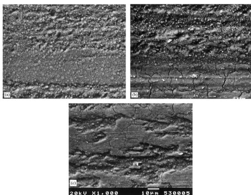
Fig. 6 SEM of the wear surfaces under different loading conditions, 1000: (a) typical wear surface after 5 N sinusoidal loading, (b) typical wear surface after 5N static loading, (c) typical wear surface after 15N sinusoidal loading.
