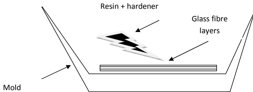
**Figure 1: The hand lay-up method**
