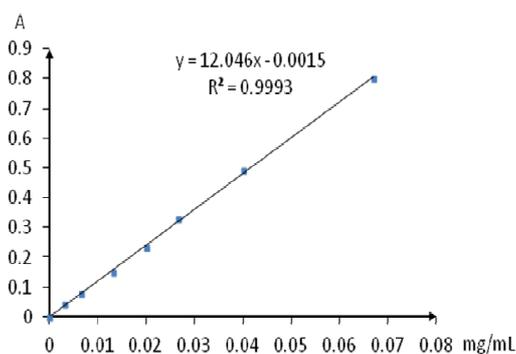
**Fig.1** Calibration plot for flavonoid determination using  $\text{NaNO}_2\text{-Al(NO}_3)_3$  method
