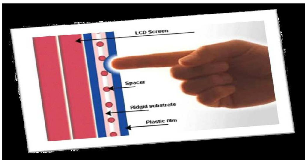
When a user touches the surface, the system records the change in the electric current that flows through the display.
