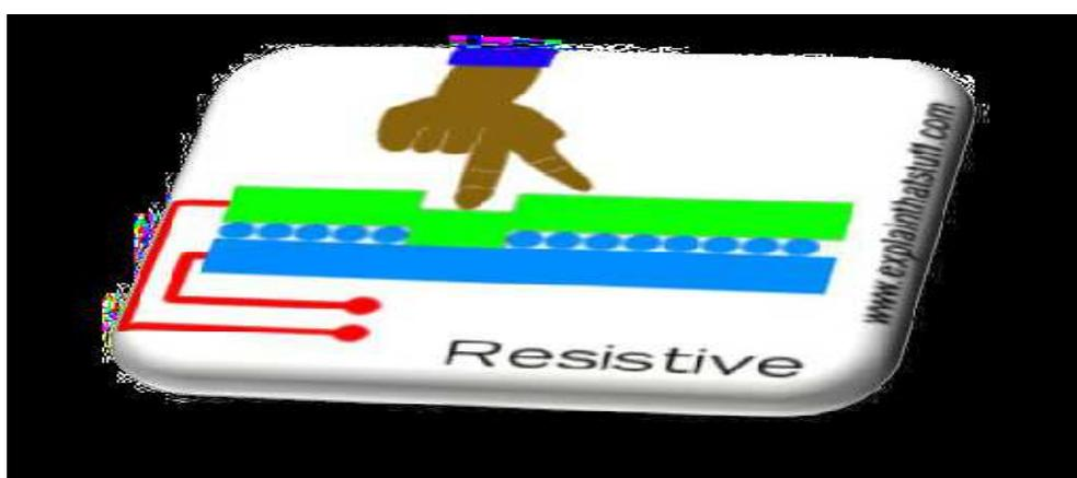
Resistive touch is used in restaurants, factories and hospitals due to its high resistance to liquids and contaminants. A major benefit of resistive touch technology is its low cost. Additionally, as only sufficient pressure is necessary for the touch to be sensed, they may be used with gloves on, or by using anything rigid as a finger substitute. Resistive touch screens suffer from poorer contrast; it can be damaged by sharp objects.
