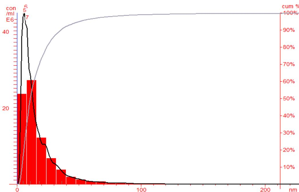
Size Distribution: Mean: 18 nm, Mode: 6 nm, SD: 24 nm. Drift Velocity: 2026 nm/s
