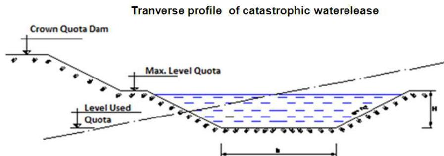
Figure 2. A transverse profile of the arrester type of channel catastrophic levels associated with filling with water
