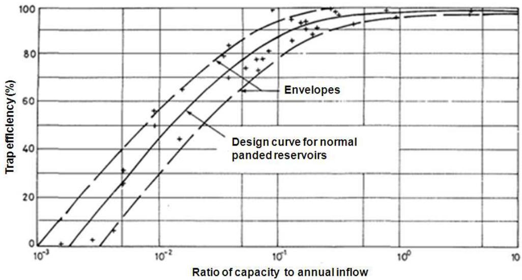
Figure 3. Determination of sediment deposited in the function of reservoir capacity report and annual flow entering in reservoir under Brunet curve (1953)
