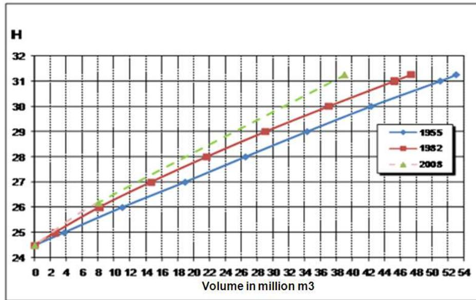
Figure 5. Graph of the water volume over releasing water
