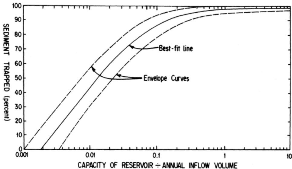
Figure 3. Graph of determination for stored sediments in function of the capacity report and annual flow for Thana reservoir
