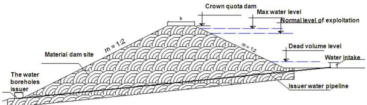
Figure 1. The dam cross section of the Thana reservoir
