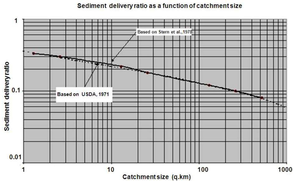
Figure 4. Determining graph of the ratio of sediment transport SDR
