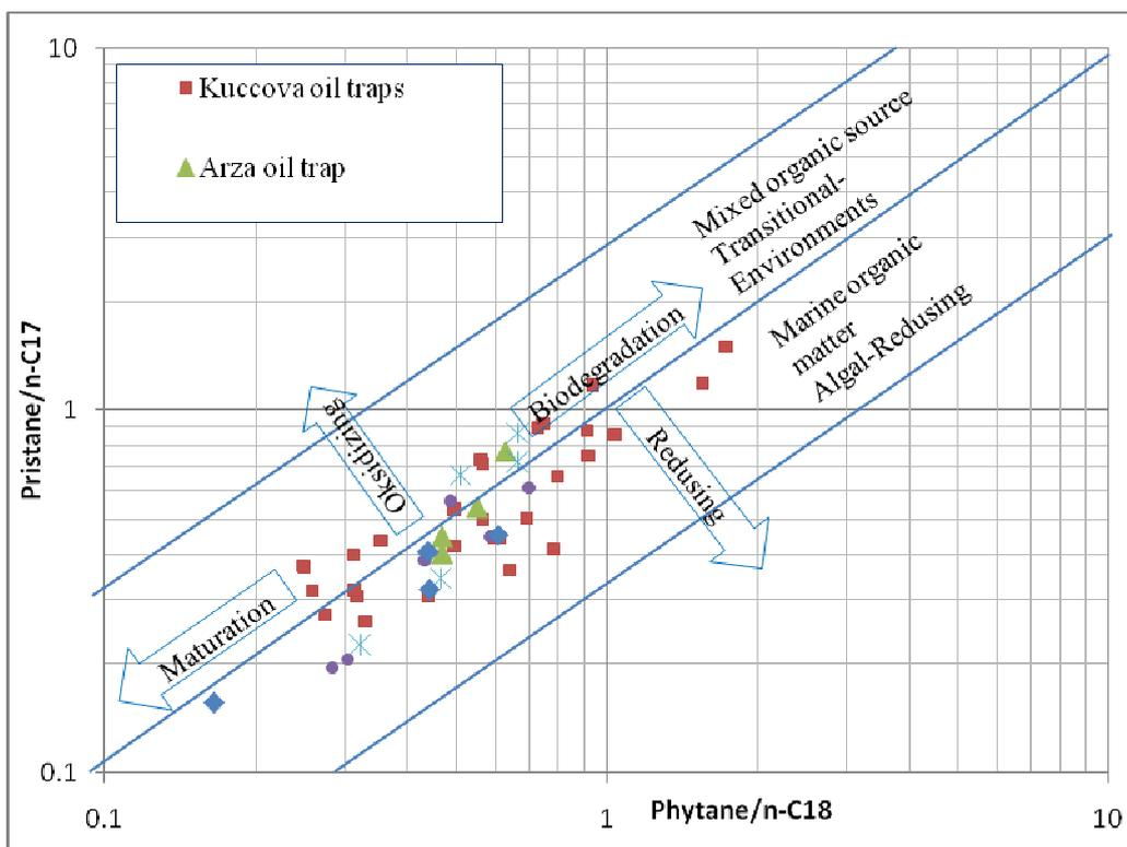
Figure 8. Environmental sedimentation of source rocks based on hydrocarbon isoprenoids (Source: Prifti & Muska ,2013; Aldahik, 2010)
