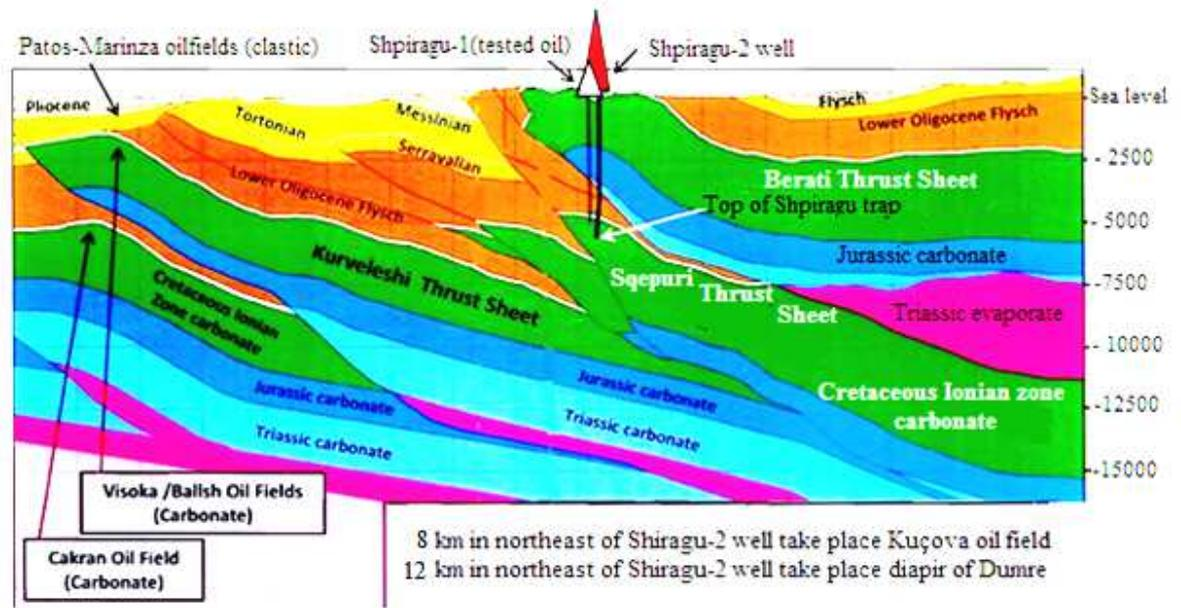
Figure 12. Cross section on Shpiragu anticline (source: [www.petromanas.com](http://www.petromanas.com))
