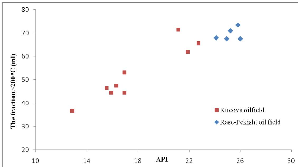
Figure5. Relations of Engler distillation vs API of crude oils in the region of Kuçova (source: Prifti & Bitri 1999).
