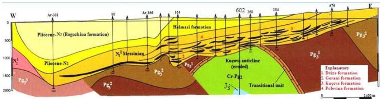
Figure 2. Section of Kuçva oilfield (source: Gjoka *et al.*, 2002, modified by Prifti)
