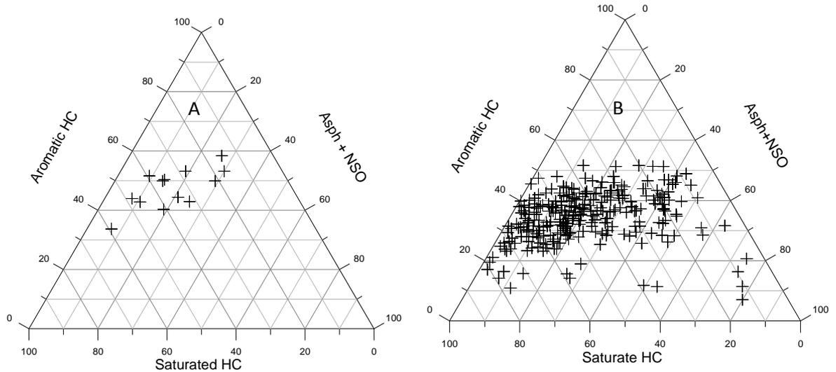
Figure 3. Triangular composition diagram of Berati anticline belt (A) and Albanian oils (B) (source: Prifti *et al.* 1999)
