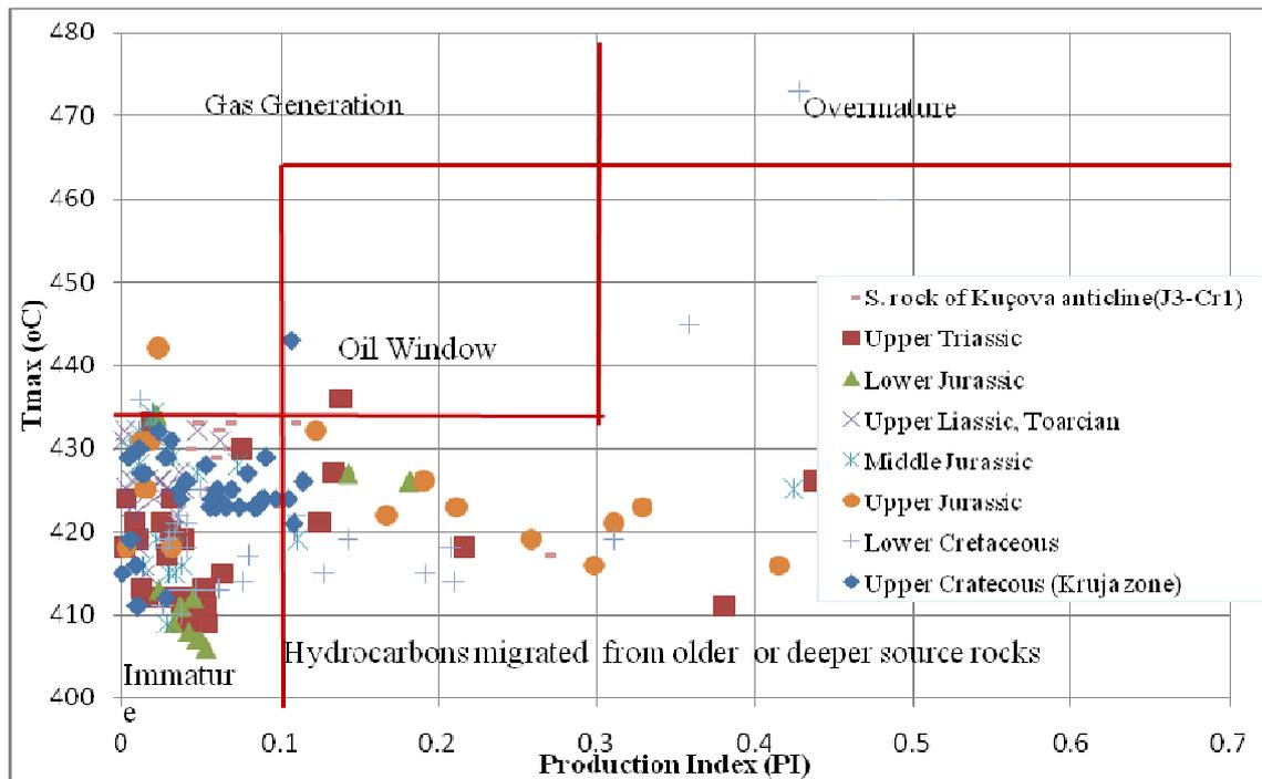
Figure 7. Maturation of source rocks based on rock-eval data (source: Prifti , based on Shiri *et al.*2013)
