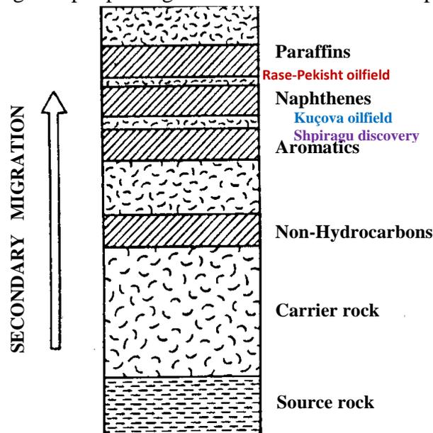
Figure 13. Separation of petroleum components during secondary migration as a result of chromatographic effects (source: Rondeel, 2001; modified by Prifti)
