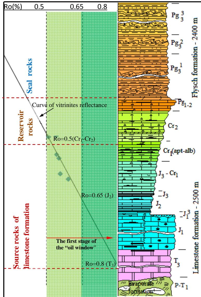
Figure 9. Model of oil generation based on vitrinite reflectance of Kuçova anticline (source: prepared by Prifti)
