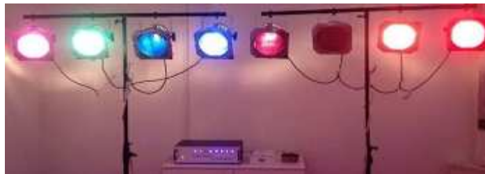
Figure 2: Neuro-Upper: the hardware system equipped with LED and the visual stimulation device used in the present study
