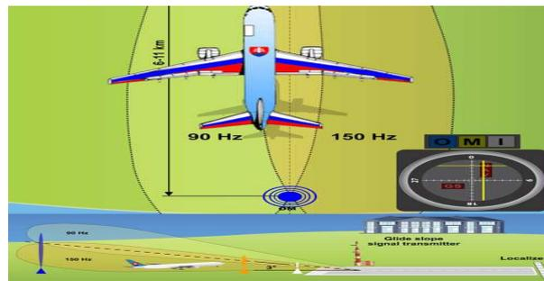
**Figure 16.** A case when the aircraft is located left of the runway's axis and too low under the glide slope.
