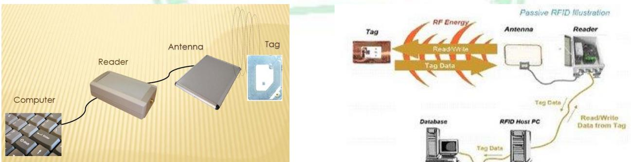
Figure No. 9.1 Diagram of RFID Working Process
