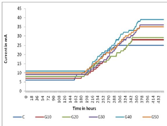
Fig 6 corrosion initiation time
