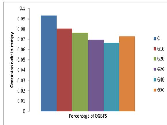
Fig 7 Corrosion rate
