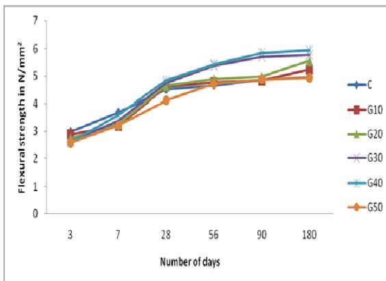
Fig 3. Flexural strength
