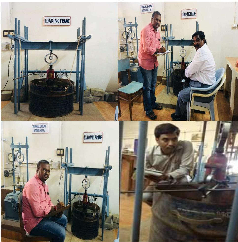
Plate 2 Author is conducting cyclic plate load test
