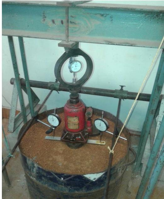
Plate 1 Experimental set up for conducting cyclic plate load test
