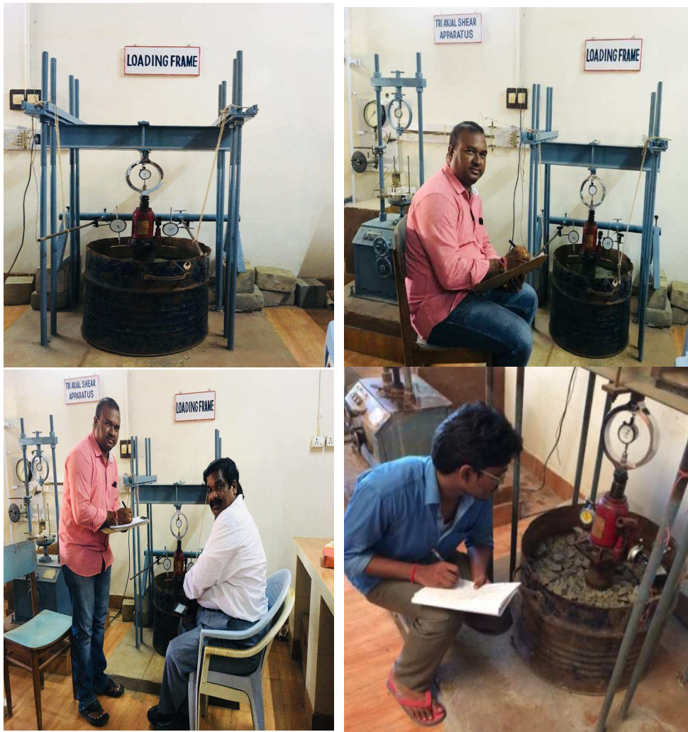
Plate 3 Authors is conducting cyclic plate load test
