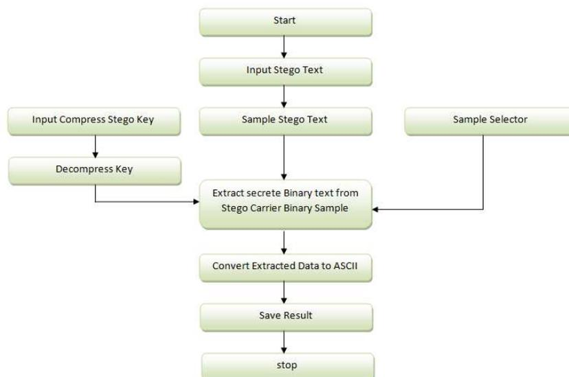
Figure 3.2.1.4 Virtual Data Extraction Block Diagram
