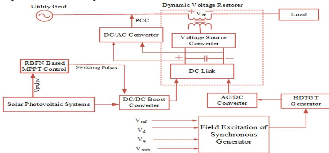
Figure 2. Solar PV, HDGT generator integration with DVR
