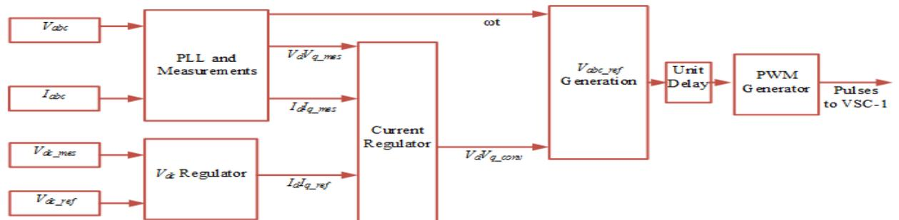
Figure 6 Control strategies of voltage source converter
