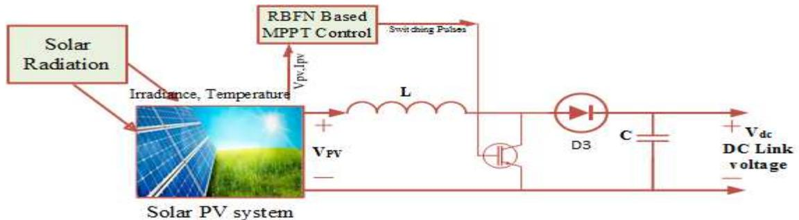
Figure 3. Solar photovoltaic systems
