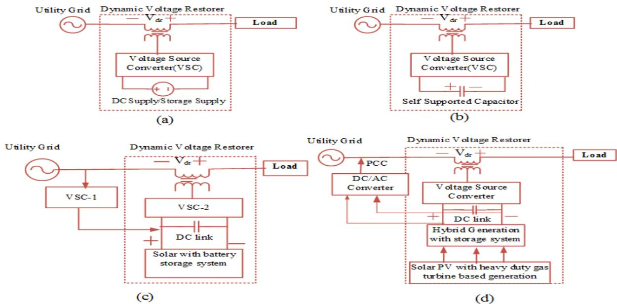
Figure 1. Dynamic voltage restorer
