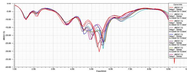
Figure 6. Optimized simulated return loss of E-slot frequency reconfigurable antenna with BAR6304 PIN diode at F4
