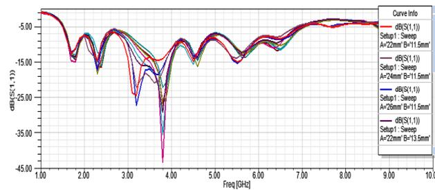
Figure 9. Optimized simulated return loss of E-slot frequency reconfigurable antenna with MPP4203 PIN diode at F2
