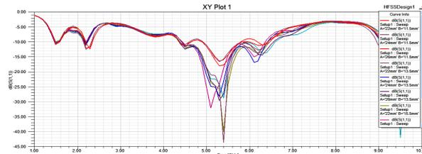
Figure 4. Optimized simulated return loss of E-slot frequency reconfigurable antenna with BAR6304 PIN diode at F2
