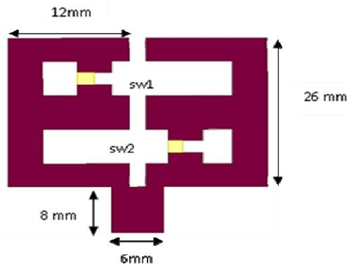
Figure 2. Geometry of E-slot frequency reconfigurable antenna with MPP4203 PIN diode
