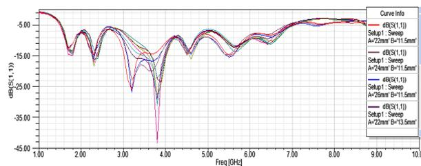
Figure 8. Optimized simulated return loss of E-slot frequency reconfigurable antenna with MPP4203 PIN diode at F1
