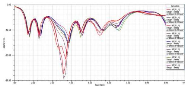
Figure 3. Optimized simulated return loss of E-slot frequency reconfigurable antenna with BAR6304 PIN diode at F1
