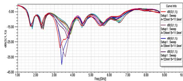
Figure 10. Optimized simulated return loss of E-slot frequency reconfigurable antenna with MPP4203 PIN diode at F3
