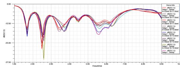
Figure 5. Optimized simulated return loss of E-slot frequency reconfigurable antenna with BAR6304 PIN diode at F3
