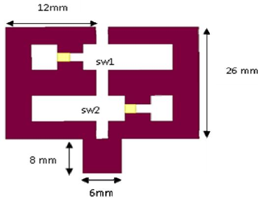
Figure 1. Geometry of E-slot frequency reconfigurable antenna with BAR6304 PIN diode
