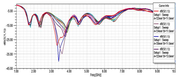
Figure 11. Optimized simulated return loss of E-slot frequency reconfigurable antenna with MPP4203 PIN diode at F4
