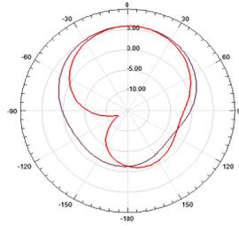
Figure 7. Optimized simulated radiation pattern of E-slot frequency reconfigurable antenna with BAR6304 PIN diode at F2
