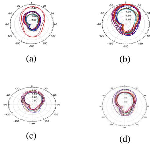
Figure 12. Optimized simulated radiation pattern of E-slot frequency reconfigurable antenna with MPP4203 PIN diode at (a)F1(b) F2 (c) F3 (d) F4
