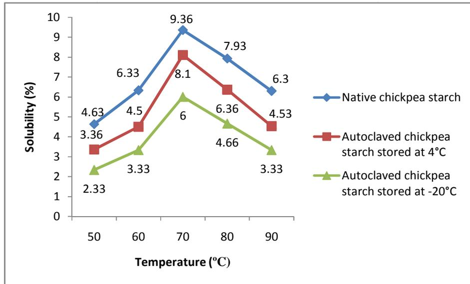
Figure 2 – Solubility of native chickpea starch and autoclaved chickpea starches stored at 4°C and -20°C submitted to heat from 50 to 90°C.
