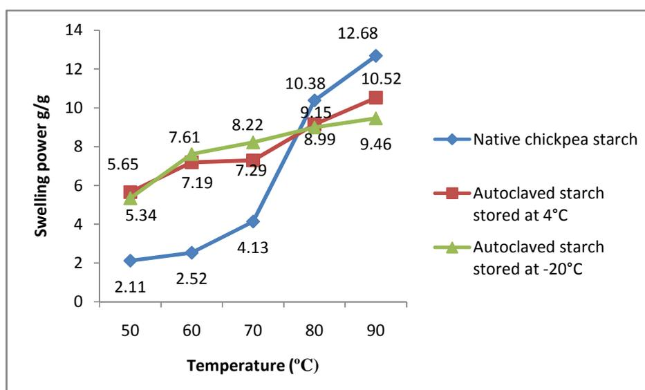
**Figure 1 – Swelling power of native chickpea starch and autoclaved chickpea starches stored at 4°C and -20°C submitted to heat from 50 to 90°C.**
